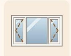
COMBINATION Opening and fixed sashes together
