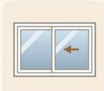
SLIDING One sash slides across
