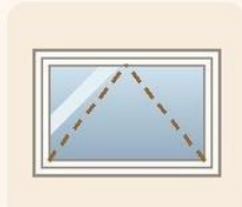
AWNING Hinged at the top, opens outward
