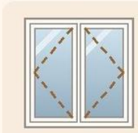
CASEMENT Cranks open from the side
